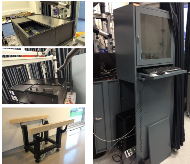
Figure 1 The SIPS prototype enclosed in the transportation box, the transportable table and vertical cabinet
