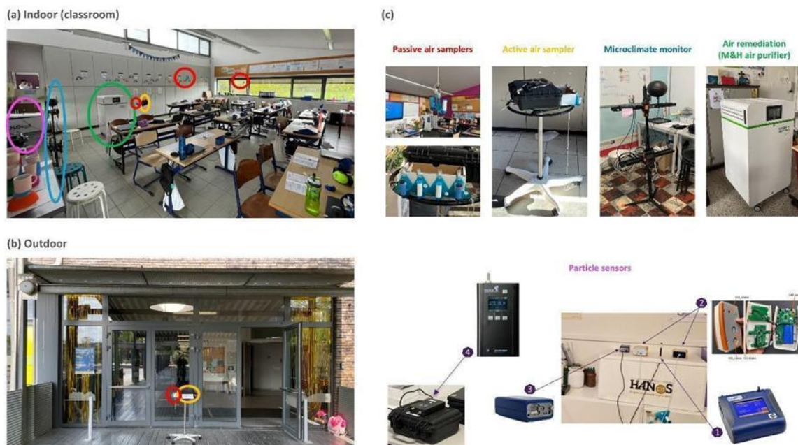
Figure 1: Overview of indoor (classrooms) and outdoor sampling settings. (a) Placement of sampling devices inside the classroom and (b) at an outdoor location. (c) Detailed view of the devices.
